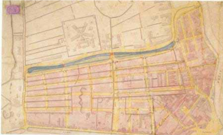
Picture 4.16 Oostblommersdijkpolder with proposed urban blocks (in pink) drawn over the polder pattern, from which the subsidence of houses can be predicted. It shows the sharp contrast between the open space and large-scale houses along the singel with the dense areas with smaller houses and streets behind it. Source: Municipal Archive Rotterdam
