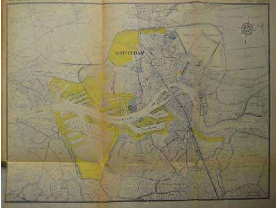
Picture 5a.8 Map of already filled in grounds in Rotterdam: Hoboken (first project hydraulically filled in), Bospolder Tussendijken and large harbour areas. Source: Commissie inzake Fundeeringen in opgehoogden Grond te Rotterdam 1931
