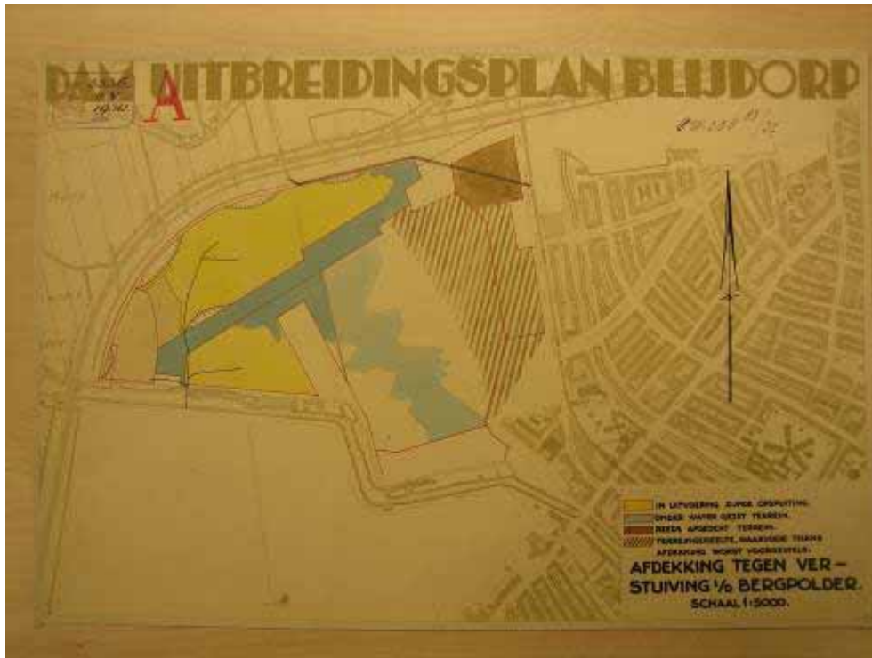
Picture 5a.25 This map belongs with a letter from the director of Public Works and shows the state of activities on 27 June 1930. The phone company complains about the sand blowing into their switchboards. The solution is to inundate the area, due to the fact that the area had irregular heights it is difficult to use the most common method of putting a layer of mud on top or grow grass.
