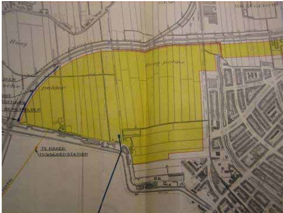
Picture 5a. 24 Technical plan of the filled area, the brown line at the north point of the Bergsingel is the new cycle connection. The red line is the (loswalkade) dike that forms the compartment that will be raised. The yellow line is the (persleiding) pipe that flushes the sand from the Driehavencomplex.
