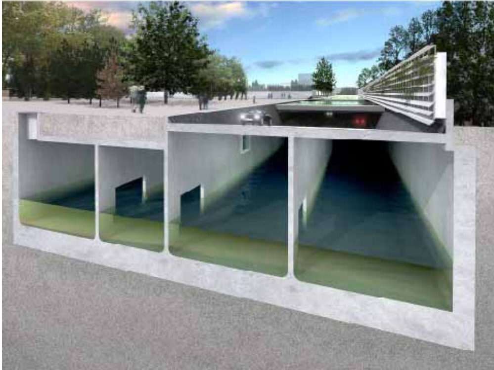
Picture 4.24 Underground parking and water storage in Rotterdam. Source: Municipal Rotterdam
