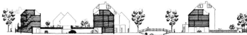
Picture 5c.3 Aerial view and cross section of Beverwaard, just like in the Jordaan in Amsterdam every other ditch is closed and the remaining widened. The back yards are lifted to create parking facilities. Source: Aeroview
