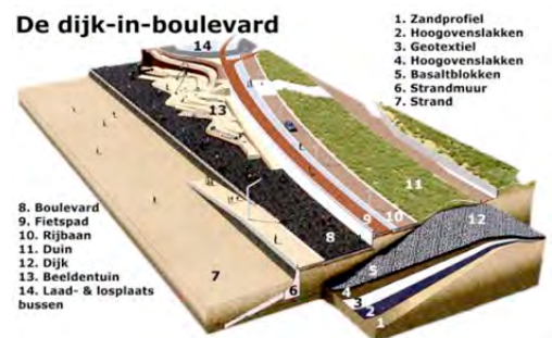
Figuur 6: De Dijk-in-boulevard in Scheveningen
