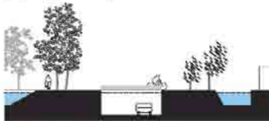
Lowering highway A9 creates a gap and requires extra security measures
