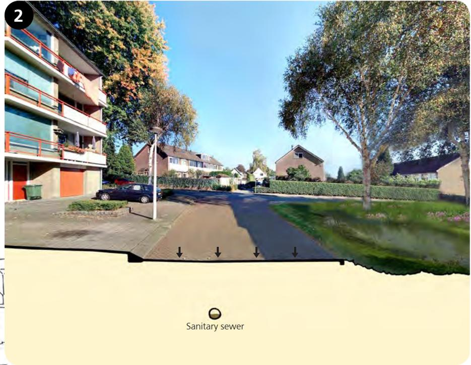
Bumps guide the water partially towards swales and partially to lower-lying area
