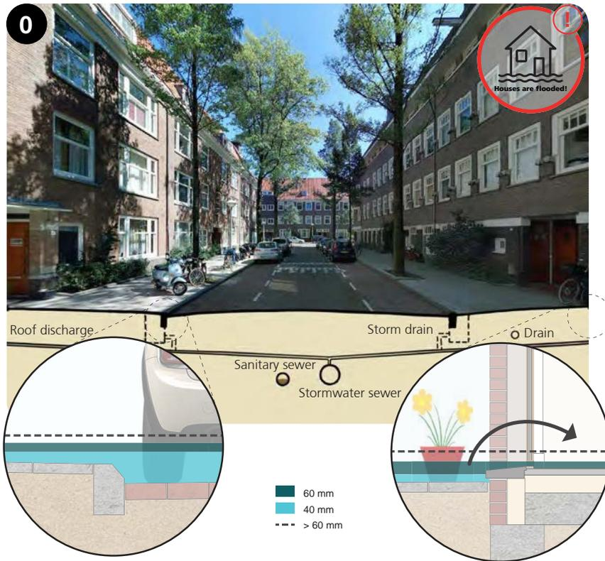
Details show water levels of 40mm, 60mm and more than 60mm in one hour
