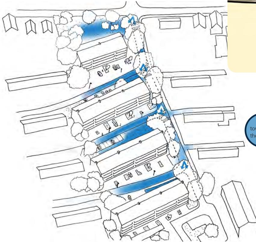
Bumps guide the water (partially) towards swales to retain the water in the area
