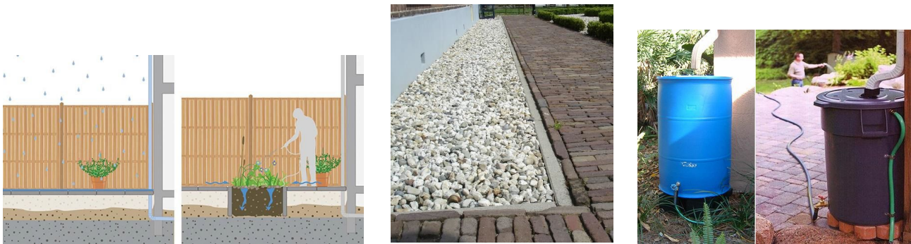
Figure 1: replacing tiles with plants + soil (left), grit to improve infiltration (middle), water barrel (right) (Boone, Braamhaar, Coppoolse, Hanning, & van Lith, 2017) (Defize, 2018)
