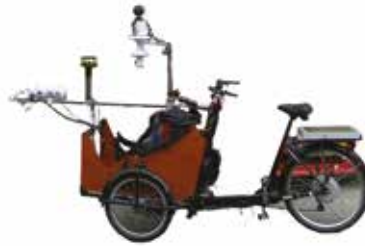
Figure 4.5: Cargo-bicycle equipped with micrometeorological measurement sensors (Heusinkveld et al., 2010)
